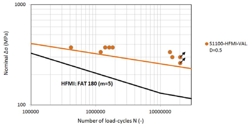
Fig. 9: Fatigue assessment of data set #3 (equivalent nominal stress range)
