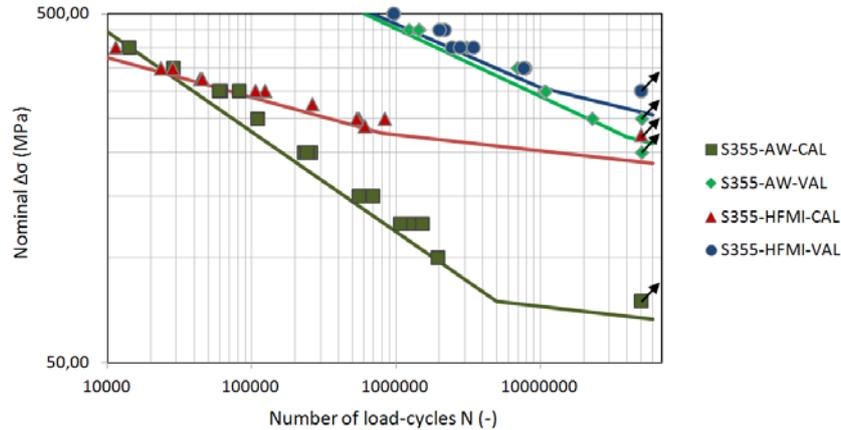
Fig. 1: Fatigue test results of data set #1 (maximum nominal stress range)
