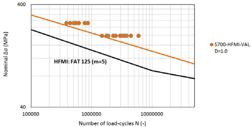
Fig. 8: Fatigue assessment of data set #2 (equivalent nominal stress range)
