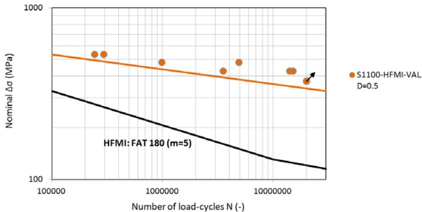
Fig. 11: Fatigue assessment of data set #4 (equivalent nominal stress range)
