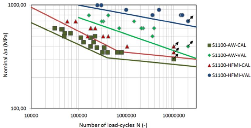
Fig. 4: Fatigue test results of data set #4 (maximum nominal stress range)
