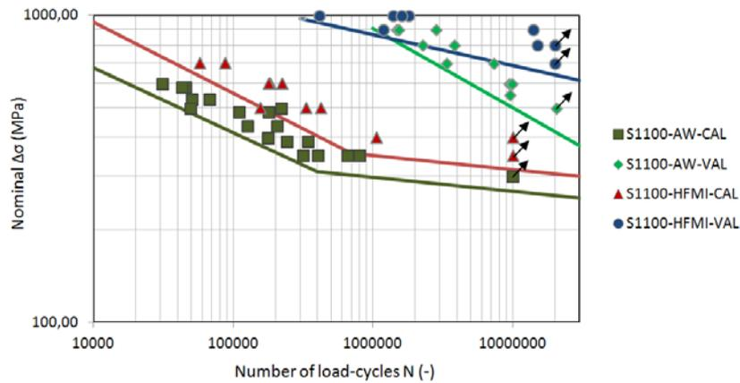
Fig. 3: Fatigue test results of data set #3 (maximum nominal stress range)
