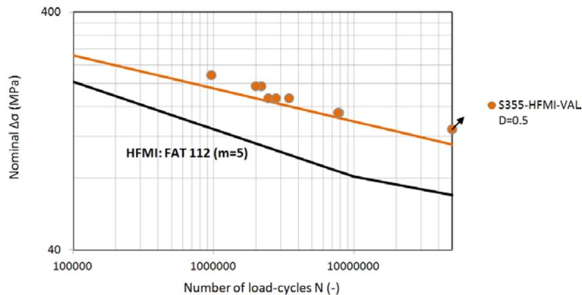
Fig. 5: Fatigue assessment of data set #1 (equivalent nominal stress range)
