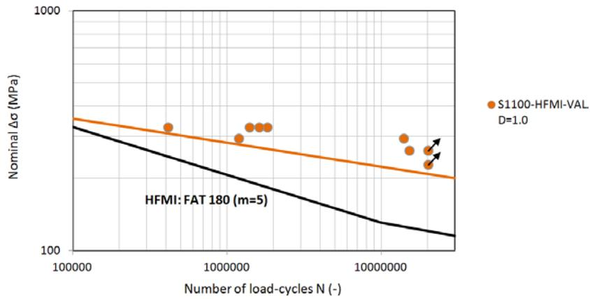
Fig. 10: Fatigue assessment of data set #3 (equivalent nominal stress range)
