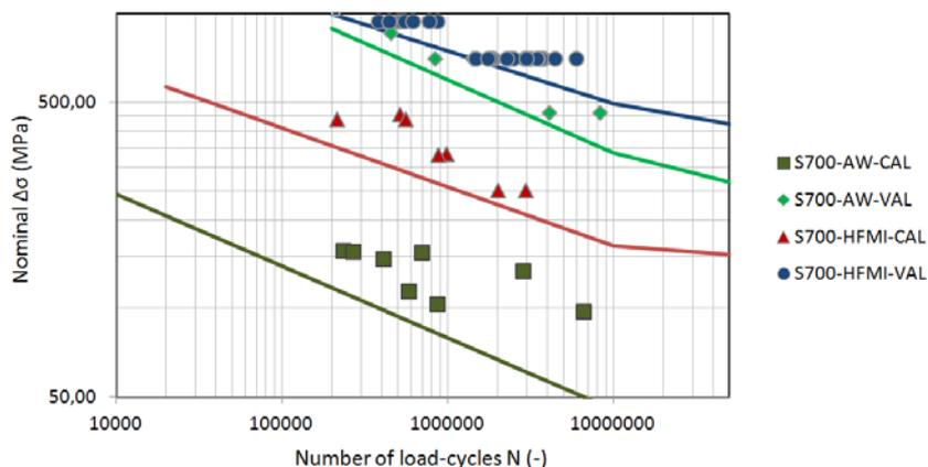
Fig. 2: Fatigue test results of data set #2 (maximum nominal stress range)
