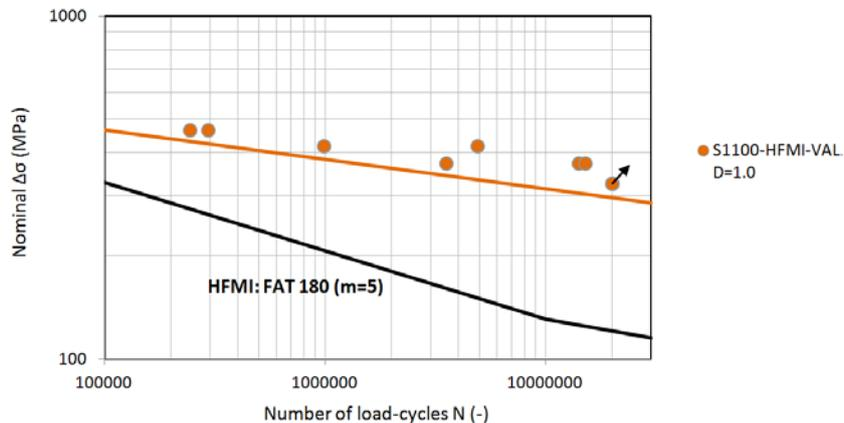
Fig. 12: Fatigue assessment of data set #4 (equivalent nominal stress range)
