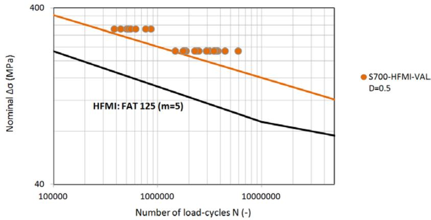
Fig. 7: Fatigue assessment of data set #2 (equivalent nominal stress range)
