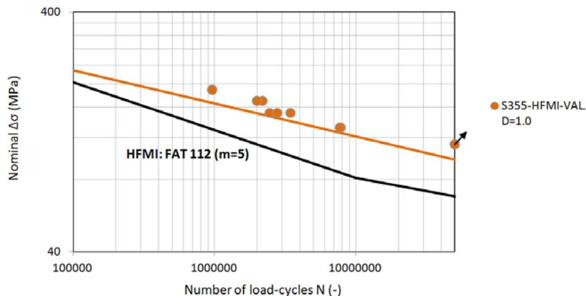
Fig. 6: Fatigue assessment of data set #1 (equivalent nominal stress range)
