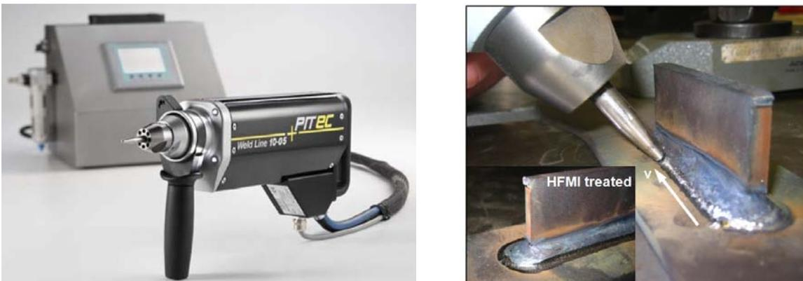
**Fig. 1:** PIT-device (hand-held and control unit) and depiction of HFMI post-treatment (by PIT) at longitudinal attachment [19]
