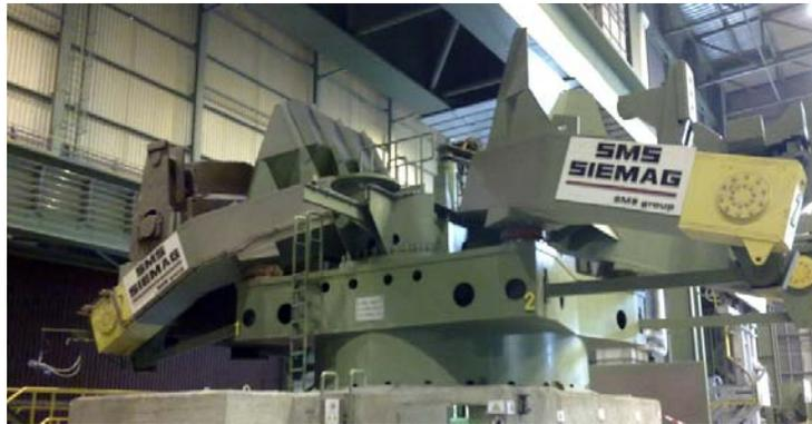
Fig. 11: Ladle turret for a continuous casting machine
