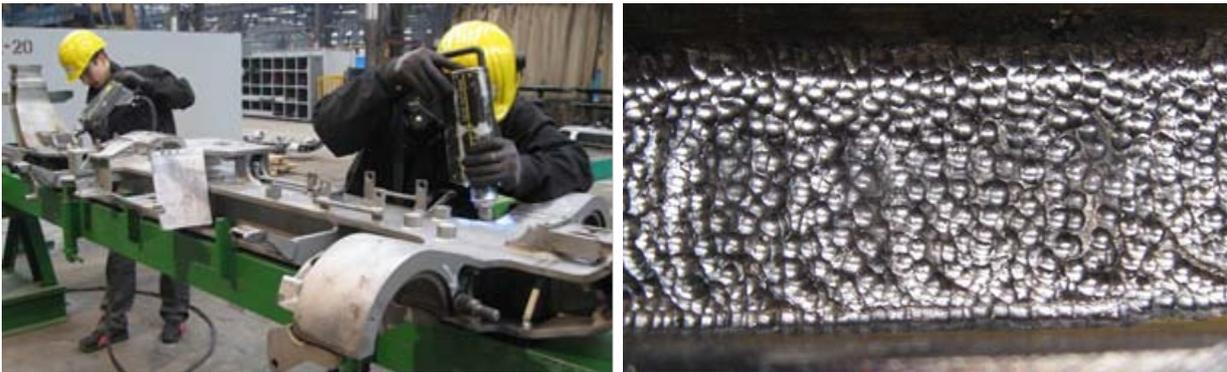
**Fig. 13:** PIT treatment of a steel frame and treatment after each weld layer
