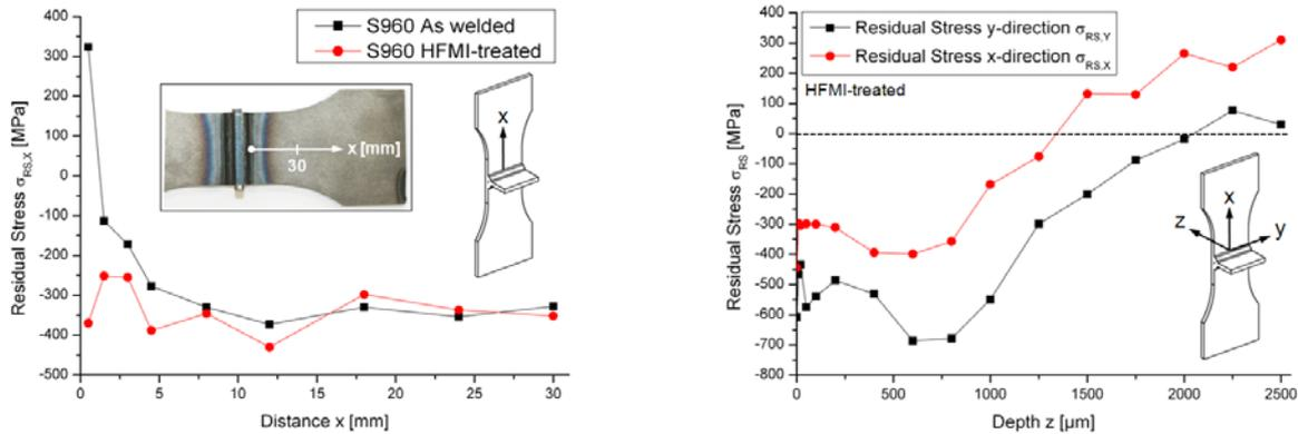
**Fig. 3:** Residual stress distributions on surface layer (left) and in depth at the weld toe (right) for high-strength S960 T-joint [24]
