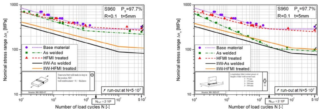
**Fig. 4:** Fatigue test results for high-strength S960 butt joint (left) and longitudinal attachment (right) [25]
