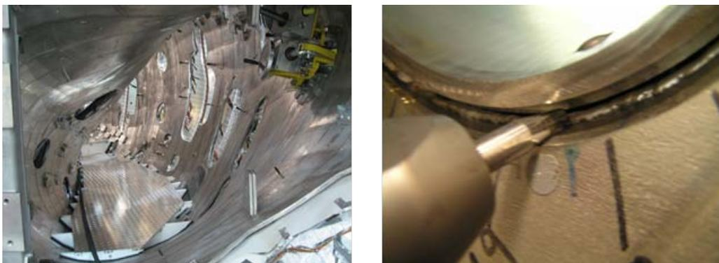
**Fig. 10:** Plasma inner shell and deformation of buffer layer
