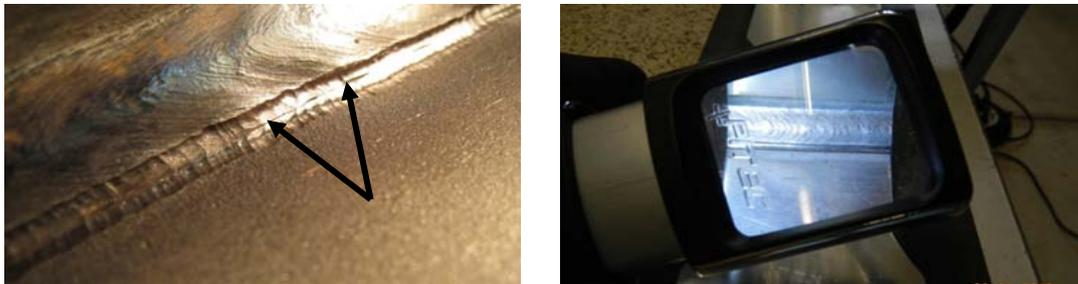
**Fig. 6:** Remaining notch of treated groove and magnifier for better recognisability
