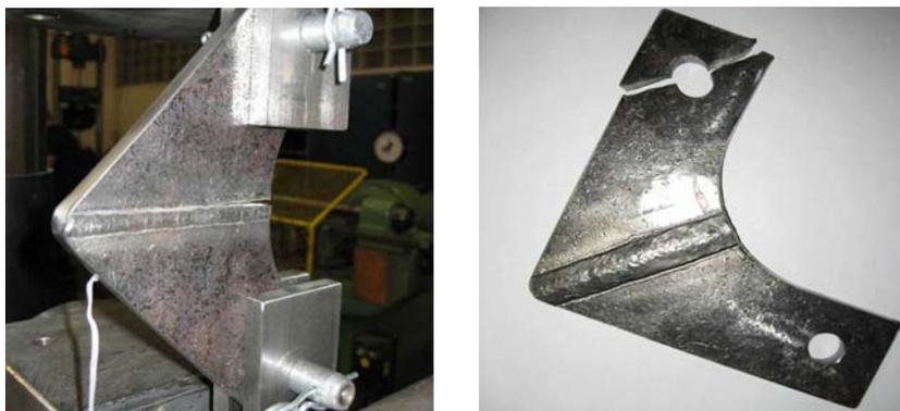
Fig. 12: Crack at 153,000 and failure at clamping after 417,000 load cycles
