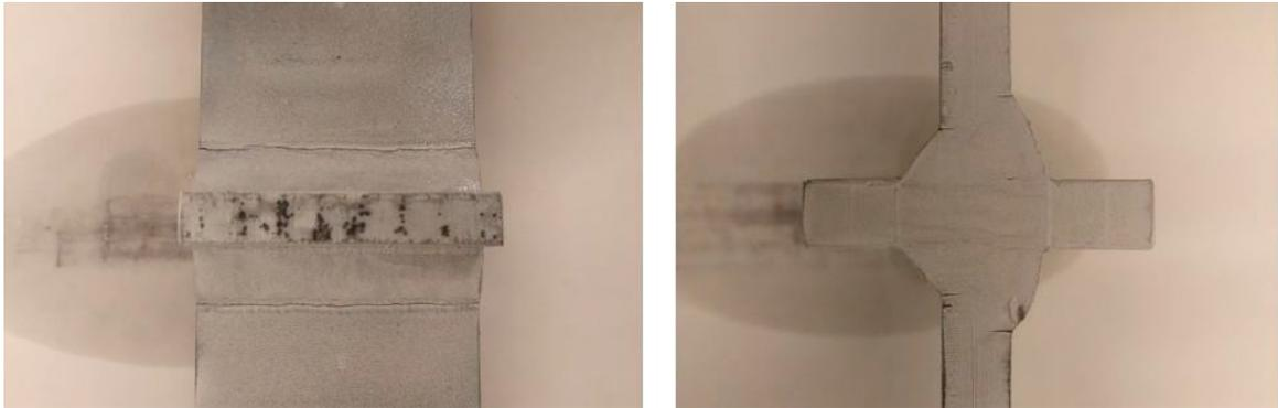
Figure 3: Typical failure mode with crack initiation at the weld toe
